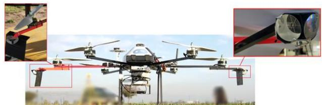
Figure 2. The UAV with the bar and the focus on the two prisms.
