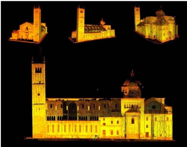
Figure 4\_The complete point cloud after registration.
