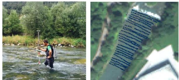
Figure 5. Field observations using RTK GPS to record water depths and location of SAVs in the Sarca River.
