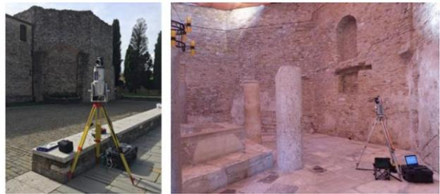
Figure 12. Acquisition of the external and internal part using TLS
