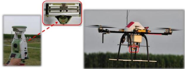
Figure 1. The retro-reflector on-board and the track with the Total Station.
