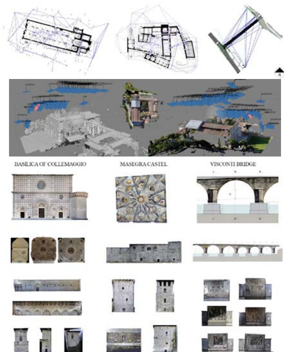
Figure 3 – Geodetic networks and digital photogrammetry data are secondary data sources used for the generation of HBIMs.
