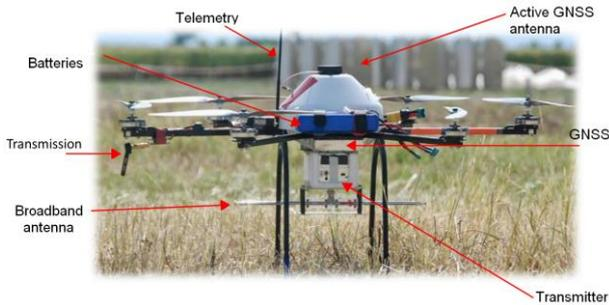
Figure 4. ArduCopter configuration for the SKA project.
