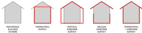
Figure 12. Explanation of building data acquired with different survey techniques
