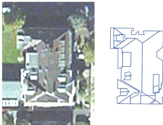
Figure 11. Results carried out over a building with a roof composed of complex slopes highlight the necessity of high density and accurate point clouds (aerial image on the left, slopes reconstructed from the point cloud on the right)
